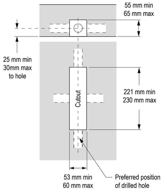
**⚠ Note:** A  $\varnothing$  20 mm min by 125 mm min deep hole must be drilled in one of four directions into the brick and as close as parallel to the wall surface as drill will allow. Antenna must fit into hole. Select direction of hole based on individual site conditions.
