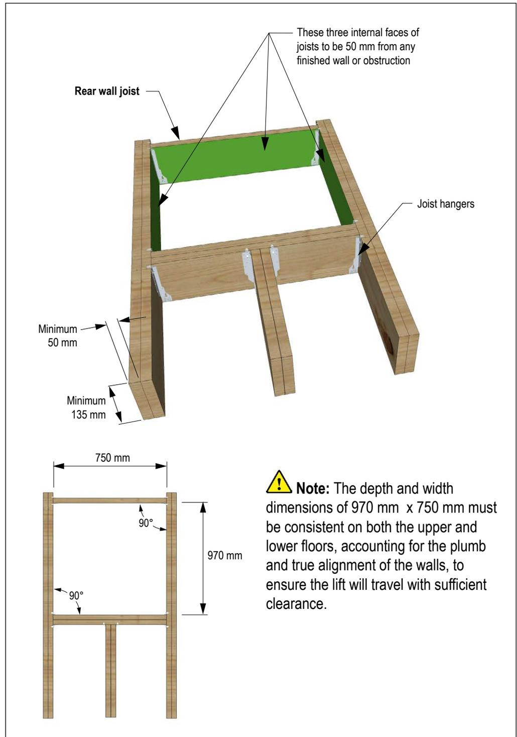
**! Note:** The depth and width dimensions of 970 mm x 750 mm must be consistent on both the upper and lower floors, accounting for the plumb and true alignment of the walls, to ensure the lift will travel with sufficient clearance.
