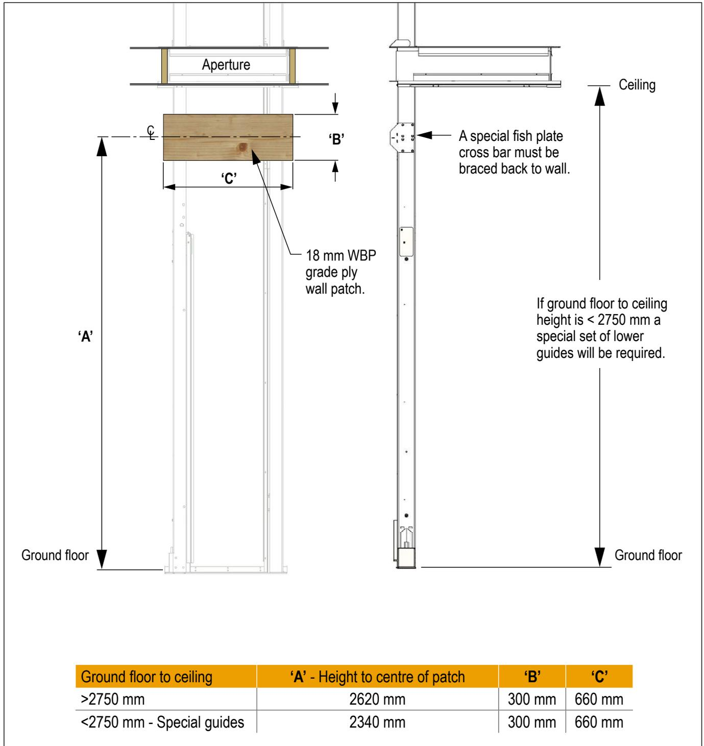
The lower guide brace kit can accommodate situations where the wall is up to 340 mm away from the rear of the aperture. If the distance is greater than this, a special bracing kit will be required.
