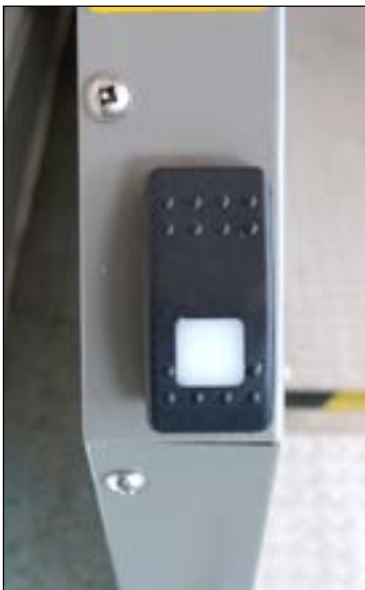
Lower level control switch (standard installation) integrated within the left hand lower level side panel
